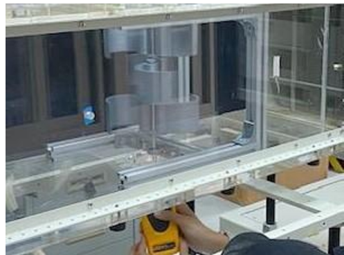
Fig. 4. Measuring rpm output reading from a Scoop Harmony VAWT [30].
