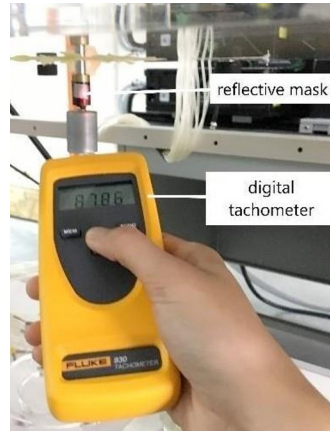
Fig. 5. Close view VAWT measurement using a Fluke 940 Digital Tachometer.
