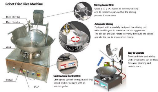
Fig. 2. Design model for the fried rice-making machine
