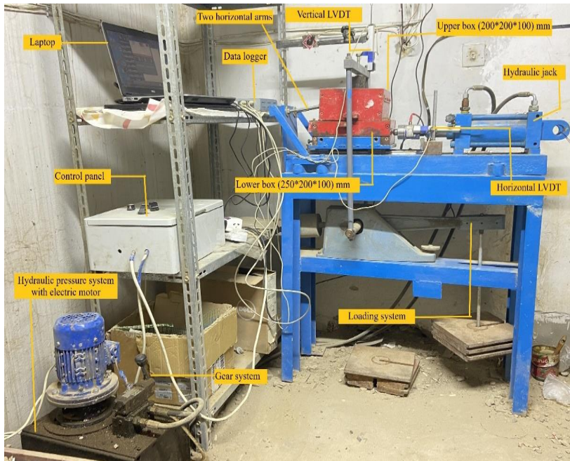
Figure 5: The large-scale direct shear device.
