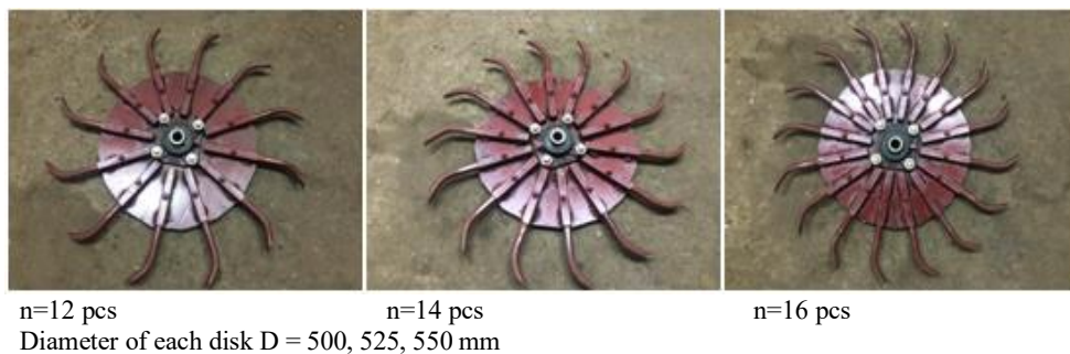
Fig. 4. Working bodies of the rotary hoe
