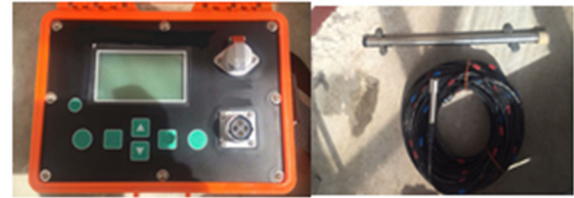
Figure 8. CX806D type foundation pit slope measuring instrument
