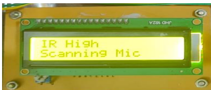
Fig. 8. Scanning of Mic after the detection of IR status
