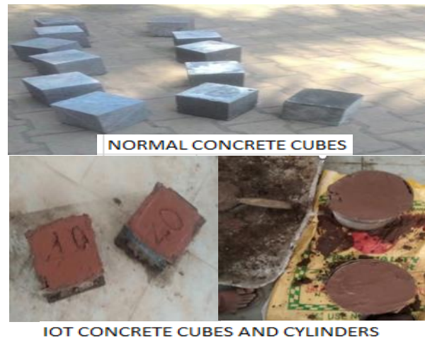
Fig: 3 Concrete & Iron ore Tailings cubes
