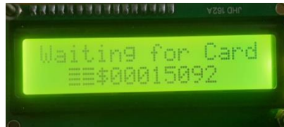
Fig. 12 LCD displaying the information for RFID tag verification
