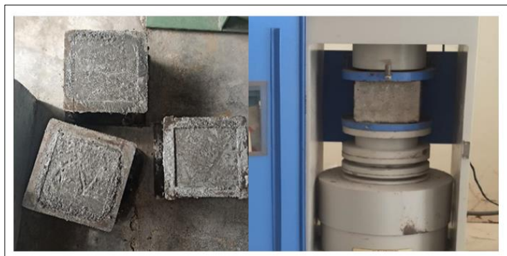
Fig 3: Cube specimen for ARGFRC-layer 1.
