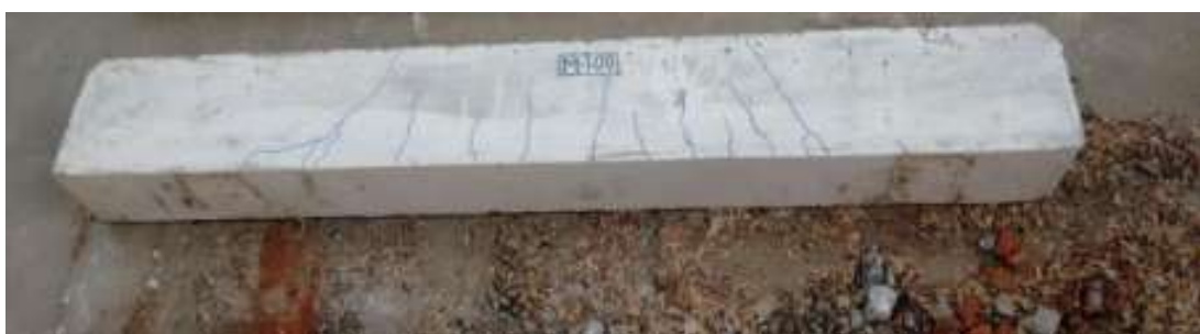
Figure 4.7 Tested D100 beam specimen
