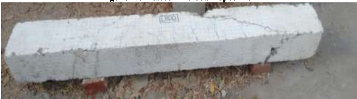
Figure 4.7 Tested D100 beam specimen
