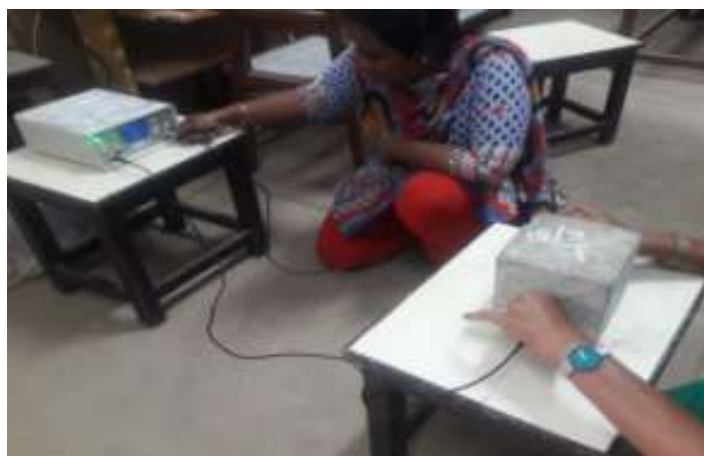
Figure 3.7 Ultrasonic pulse velocity test
