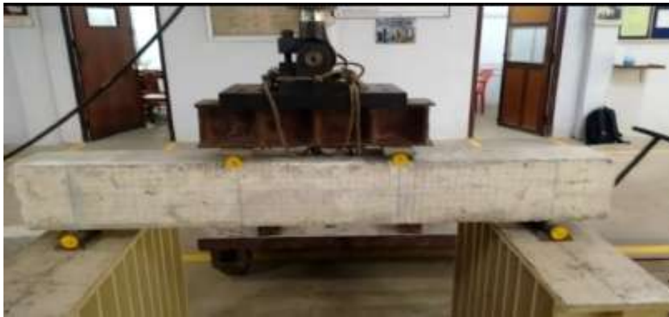
Figure 3.6 Test setup for cyclic loading
