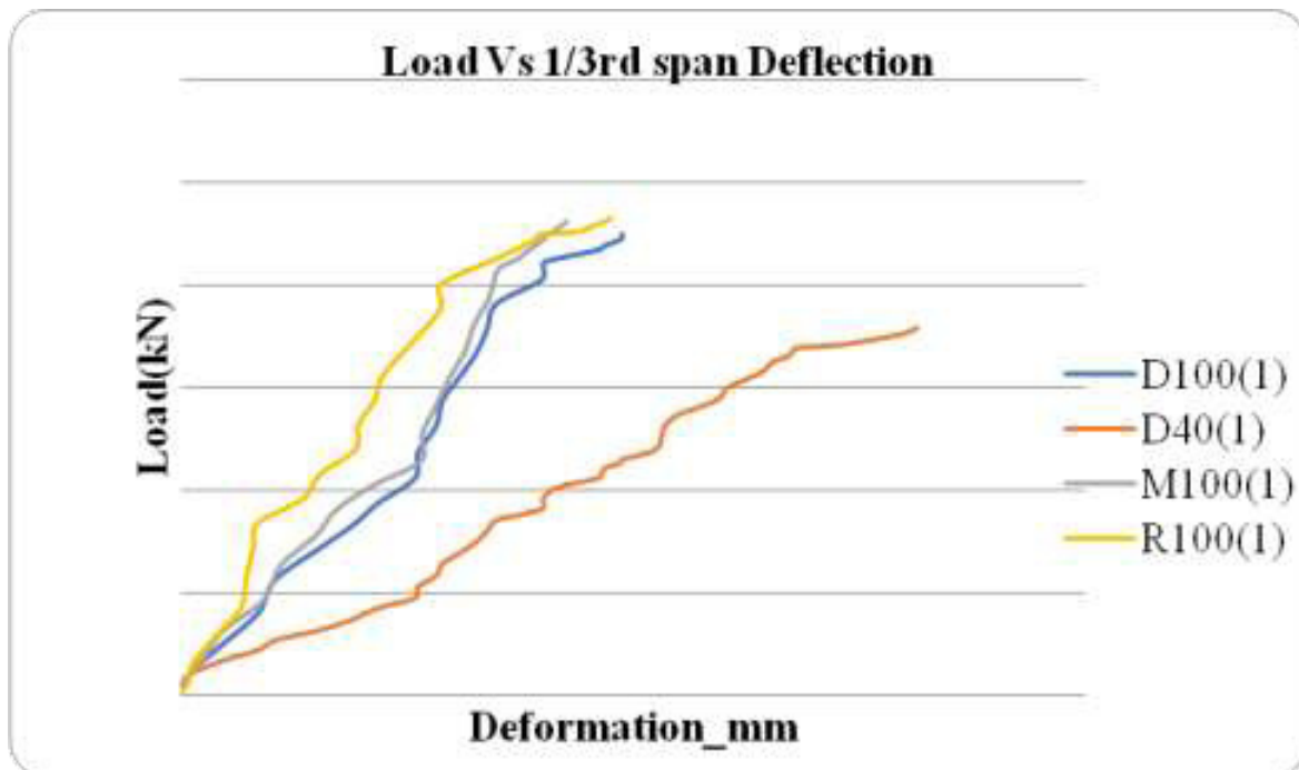
Figure 4.10 Load Vs 1/3 rd deflection
