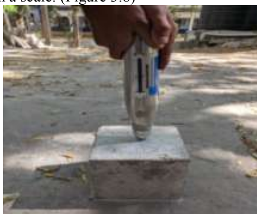
Figure 3.8 Rebound hammer test
