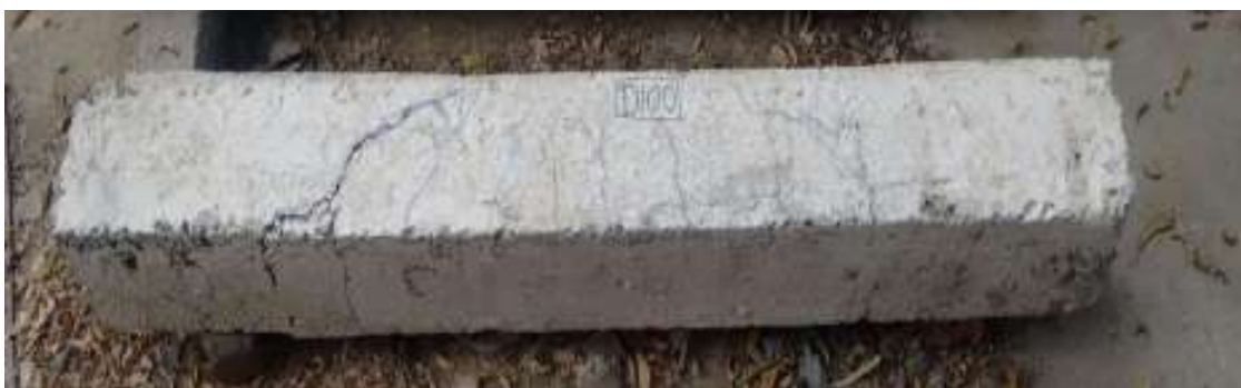
Figure 4.13 D100 beam after cyclic loading
