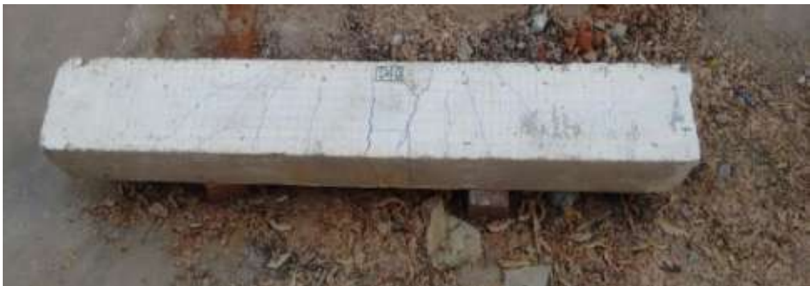
Figure 4.6 Tested D40 beam specimen
