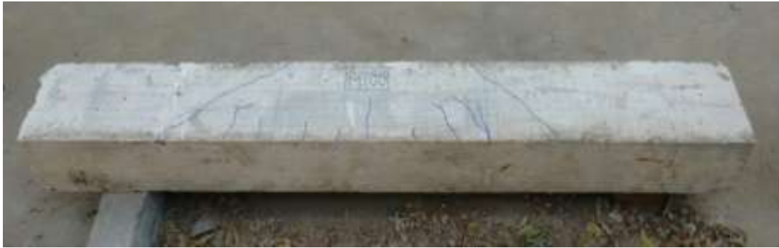
Figure 4.14 M100 beam after cyclic loading
