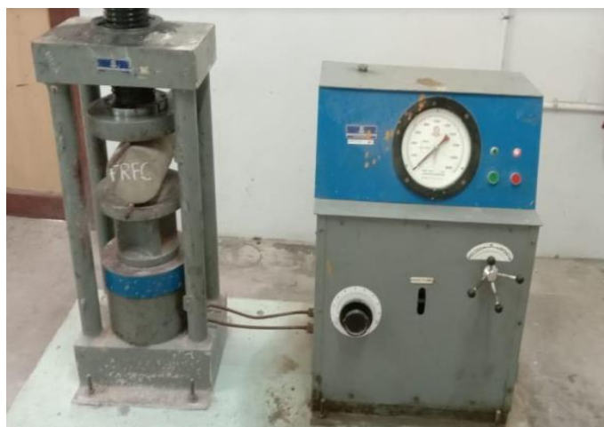
Figure 3: Testing of Cylinder Specimen
