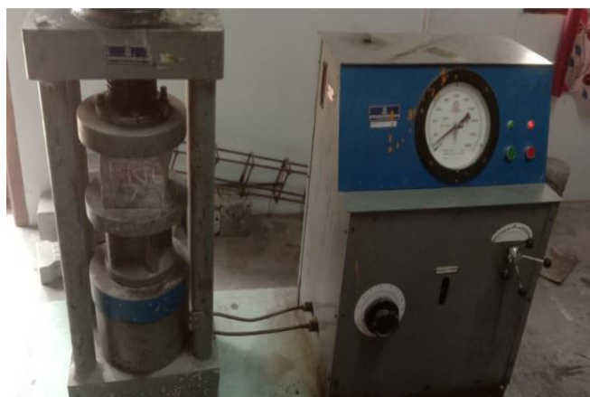
Figure 1: Testing of Cube Specimen
