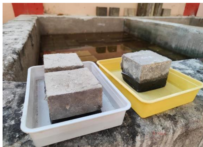
Figure. 4 Water Absorption Test
