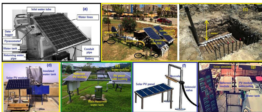
Fig.3 (a) Cooling of PV module by water cooling test rig [27] (b) Photograph of the experimental setup with BHE arrangement. [10] (c) The structure of BHE arrangement underneath. [10] (d) Front view of the PV module's experimental setup of the water-cooling system [8].(e) Experimental setup with the nozzle to cool the front surface of the PV module (PV) setup[3]. (f) Arrangement of pulsed spray water cooling setup [14]. (g) Experimental setup of cooling of PV module with water fountain [33]
