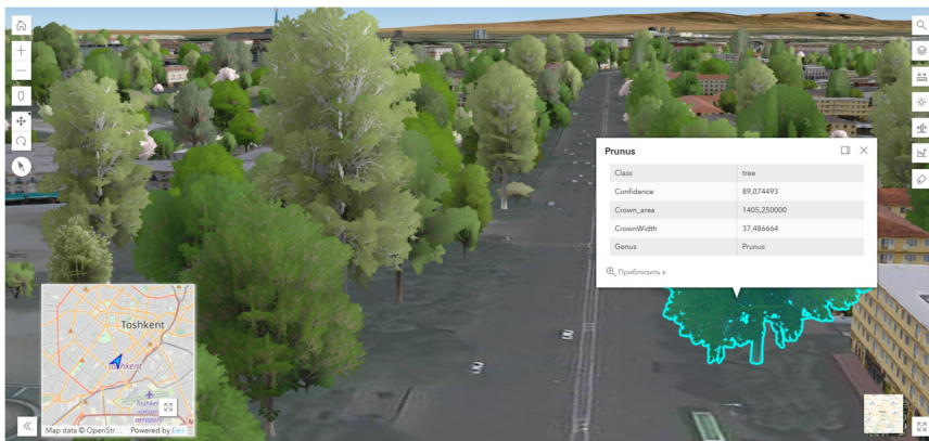
Fig. 6. All trees and vegetation were recognized and classified using machine learning.
