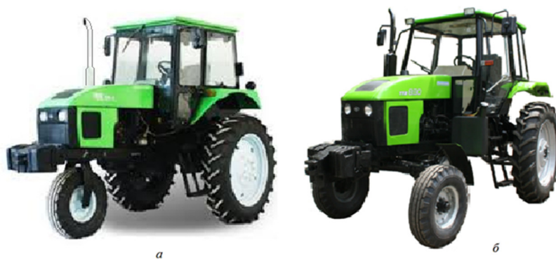
Fig. 1. Universal-tiller tractors with 3W2 (a) and 4W2 (b) wheel arrangements.
