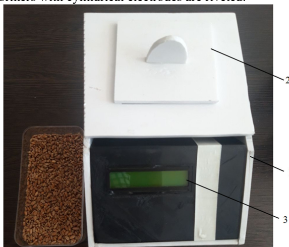
Fig. 3. The capacitance measuring device of grain and grain products: 1 is the frame, 2 is the lid, 3 is the light crystal indicator
