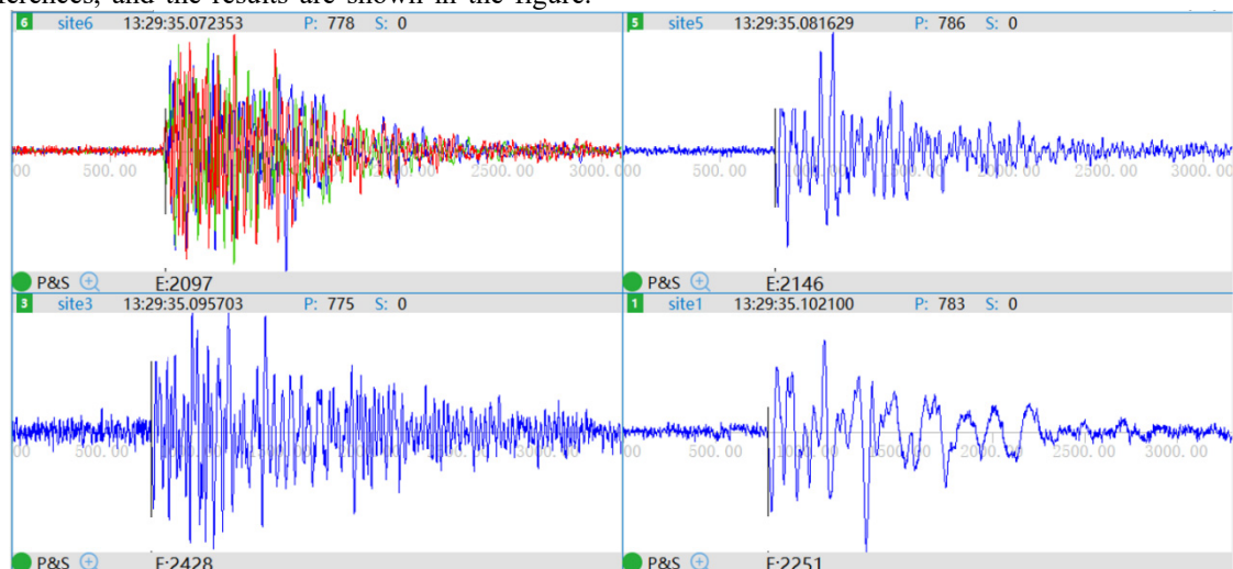
Figure 2. The microseismic signal automatically recognized by the system
