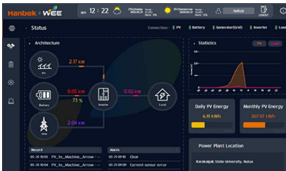
Fig.2. Main monitoring interface screen
