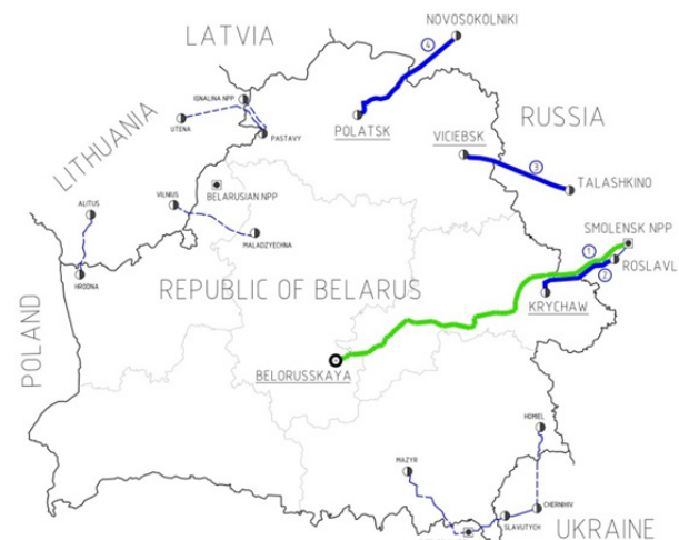
Fig. 1 330 kV and 750 kV transmission lines connecting the Belarusian power system with the UES of Russia.
