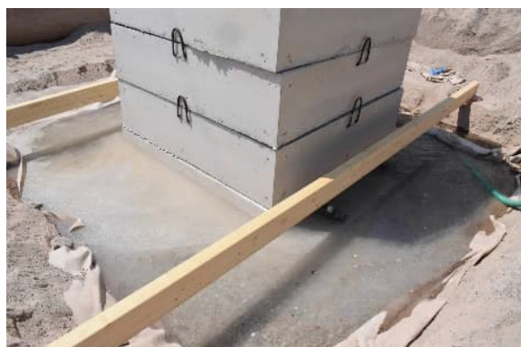
Fig. 10. Inundation of the gravel layer under constant vertical pressure.
