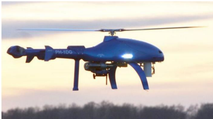
Fig. 14. Helicopter-type drone for monitoring the level of soil and water pollution.
