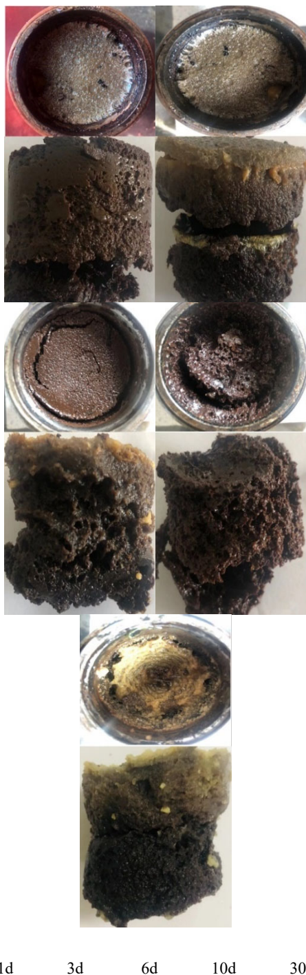
Fig. 4 Diagram of the state of gel at different times of heat treatment
