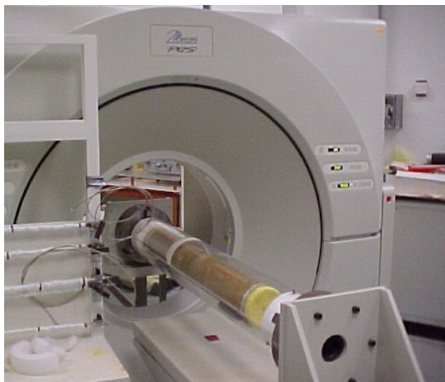
Fig. 2. Fiberglass core sleeve with rubber caps at the two ends placed concentrically in the Plexiglas housing of a converted medical CT-scanner before scanning.
