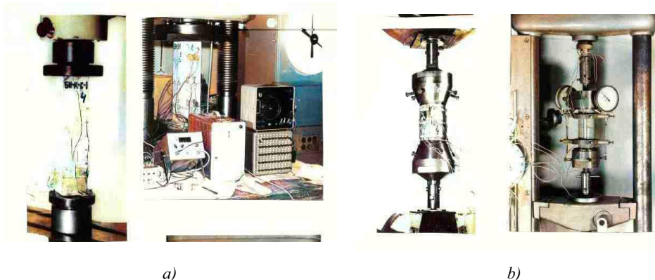
Fig. 2. Testing specimens under short-term compression ( a ) and tension ( b )
