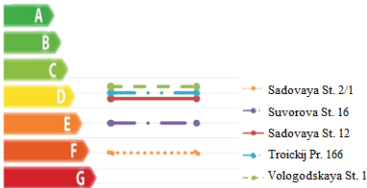
Fig. 8. Distribution of apartment buildings of series 93-012, 84 (panel) according to the energy efficiency scale.
