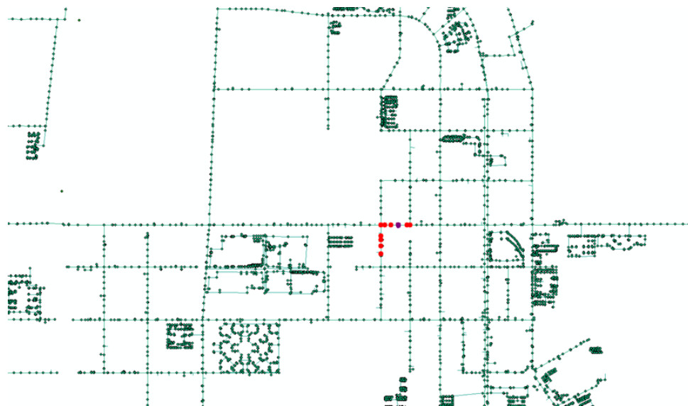
Fig. 5. Explosion accident points analyzed by pipe burst Location model and the actual explosion accident point.
