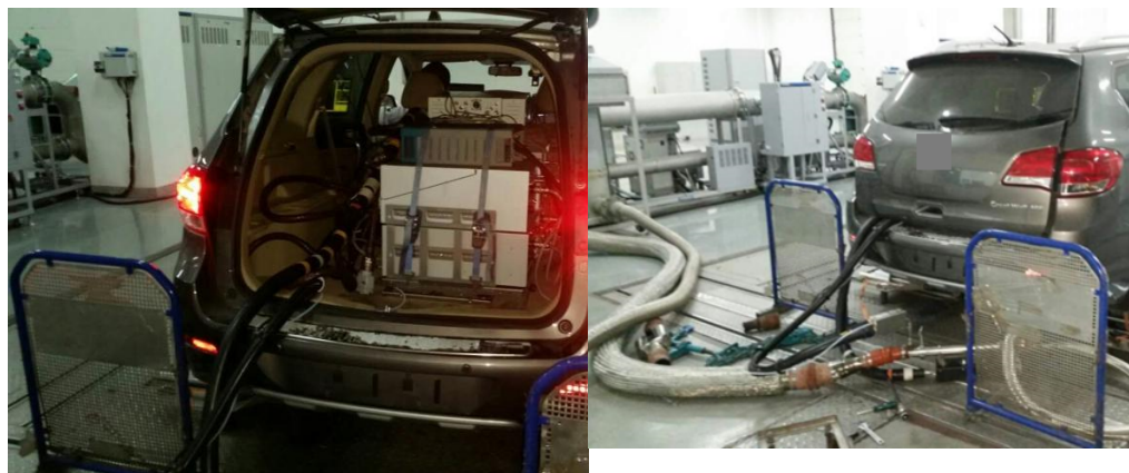
Fig. 3. The Installation statuses of PEMS verification test of vehicle 2. PEMS is in series connected to the Chassis Dynamometers system, the test cycle is WLTC cycle.
