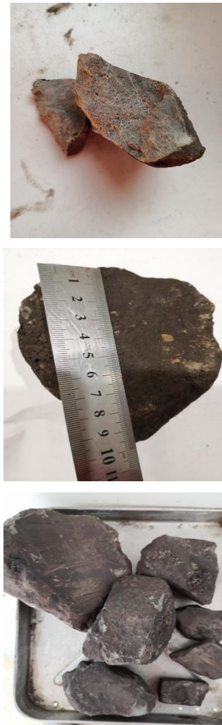
Fig. 10 The cement block returned after the first cement injection in Zhong-14 well
