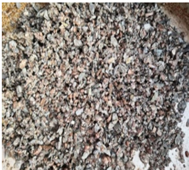
Fig. 2 Return drop during well drilling
