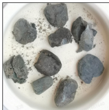
Fig. 7 Blocks of Yanchang Formation in Zhong-7 well are easily dispersed and collapsed after being soaked in water
