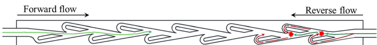
Fig. 1 Schematic diagram of fluid diode by Tesla structure [1] (flow resistance changes between forward and reverse flow)
