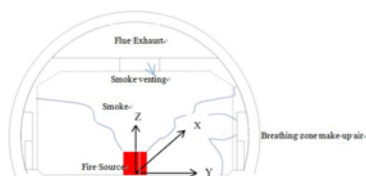
Fig. 5. Cross-sectional diagram of makeup air and smoke exhaust system
