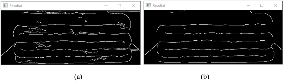
Fig. 4. Edge detection with Canny function: (a) without threshold values (b) with threshold values.
