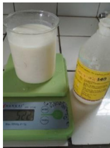
Fig. 2. The density observation of MOL by taking sample 500 ml on a digital balance
