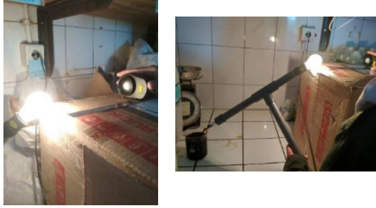
Fig. 3. The brightness value observation by dipped using soil fertility tester to conduct electricity
