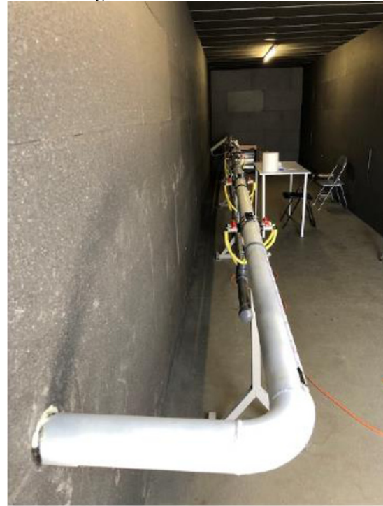
Fig. 2. Pipeline section inside the anechoic chamber
