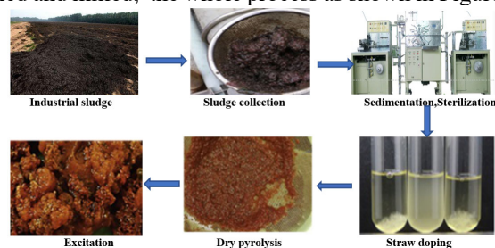
Fig. 1 Sludge scouring and purification process
