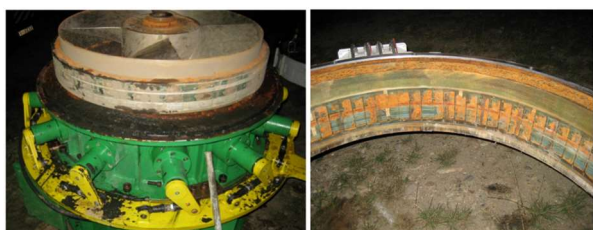
Fig. 8. An example of the influence of contaminated water on the abrasion of the composite sealing the stator and rotor in a turbine integrated with a wet gap
