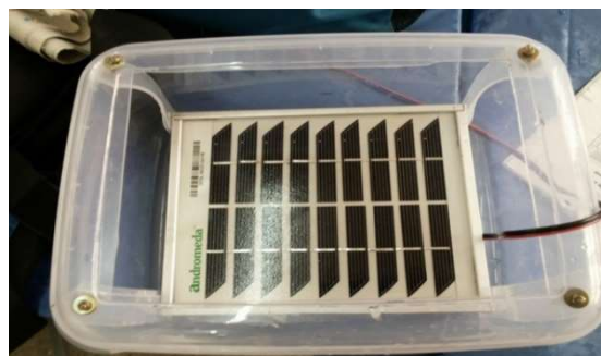
Fig. 13. PV module immersed in water [46]
