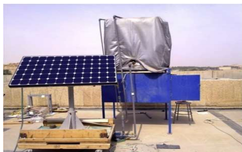
Fig. 11. Experimental setup for cooling the PV module [45]
