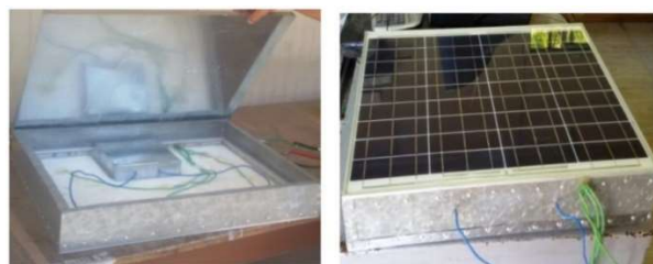
Fig. 8. a) PCM box b) PV-PCM connection [42]
