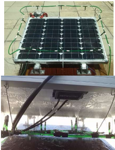
Fig. 14. The water spraying cooling of PV module [47]
