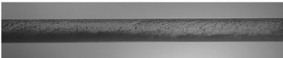
Fig. 12. The annular structure of the flow, experiment; Re_g = 28\ 000 , Re_l = 17\ 000 .
