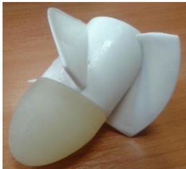
Fig. 10. Impeller designed using classic approaches.
