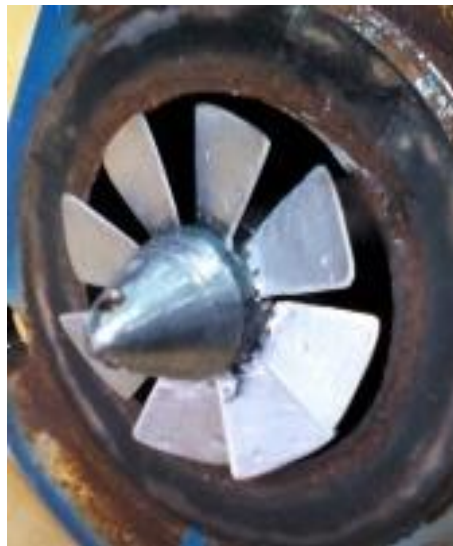
Fig. 6. Impeller designed using Nicholas E. Zhukovsky theory.
