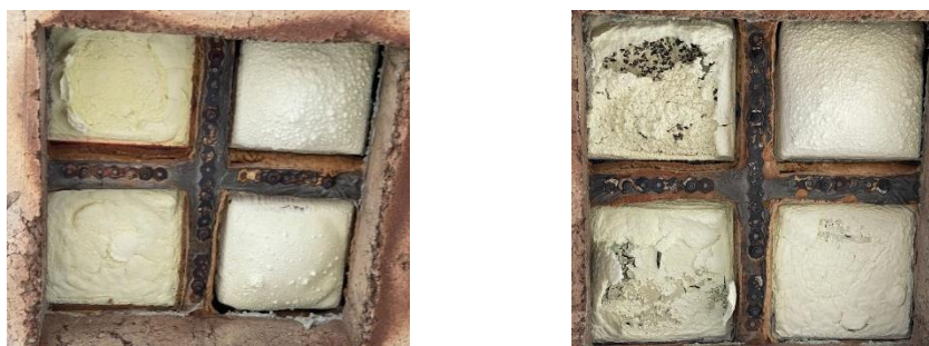
Fig. 7. Charred layers formed during fire tests; on the left – test No.1, on the right – test No.2; samples are located clockwise, starting from top left segment – IC3, IC4, IC2, IC1
