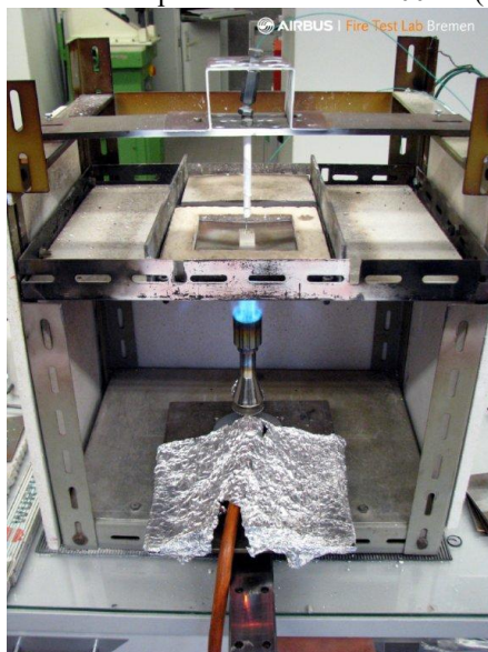
Fig. 2. Small-sized installation for fire tests of flammability of magnesium alloy samples [21]
