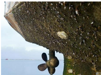
Fig. 1. Fouling of the bottom of the ship by micro-organisms
