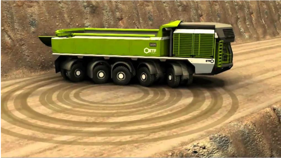
Fig. 5. General view of a dump truck with five driving axles and synchronously turning wheels to minimize the width of the turn area
