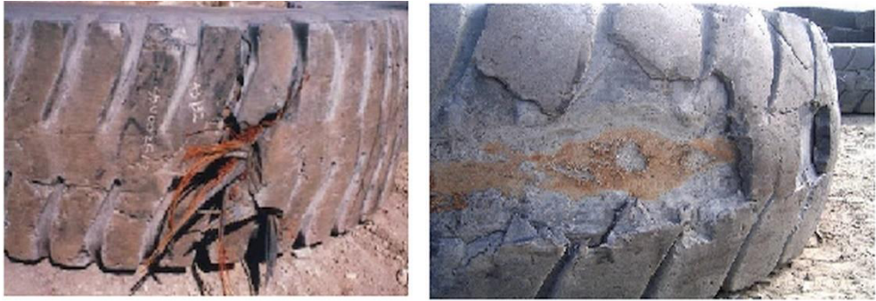
Fig. 4. Tire damage due to thermal failure.
