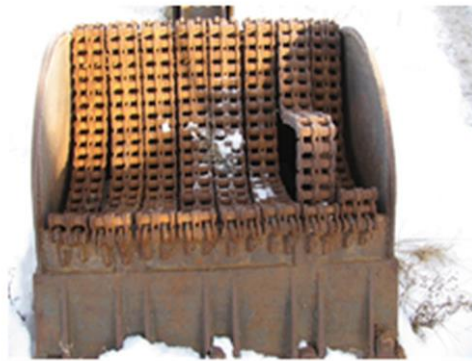
Fig. 7. The bottom of the excavator is made in the form of chains.
