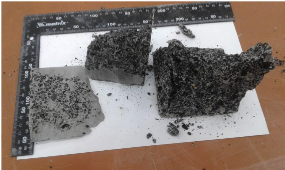
Fig. 3. Sample segregation under compressive strength testing
