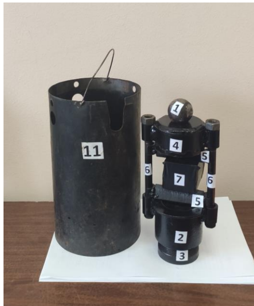
Fig. 3. Device for securing the sample before lowering it into the bucket 11
