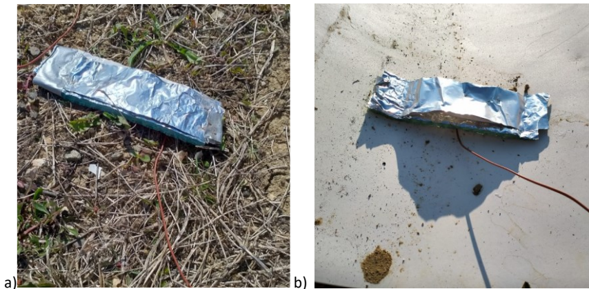
Fig. 6. Thermocouples at the ground level (Figure 6a) and at the membrane side top (Figure 6b).
