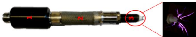
Fig.1. Representation of the streamers development produced by the corona-streamer type igniter (1=inductor, 2=connection, 3=firing-end)
