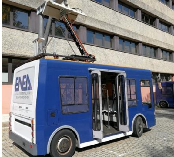
Fig. 2. Electric bus being part of the experimental test rig at ENEA Casaccia Research Center.
