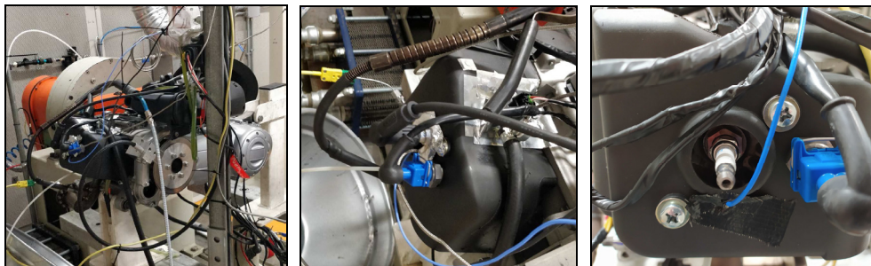
Fig. 1. Engine test-bench facility (a), LPDI injector (b), and prechamber host in the cylinder head (c).
