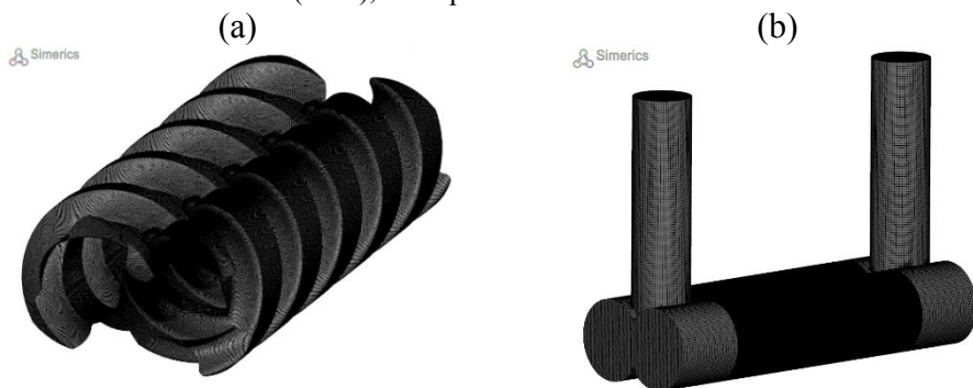
Fig. 6. Grids of the fluid domain: a) Rotor fluid domain, b) Entire fluid domain
